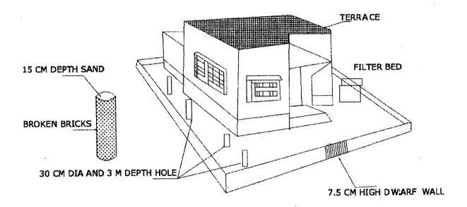
Dig a number of 3 mtr. deep and 30 cm dia percolation pits at an interval of 3 mtrs. around the plinth fill them up with broken bricks and pack the top 15 cm. with river sand. Erect 7.5 cm. high dwarf walls entrance to facilitate recharge.
